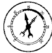
GUIDES DE SOUPAPE USES (STABLE A REGIME SUPERIEUR)
